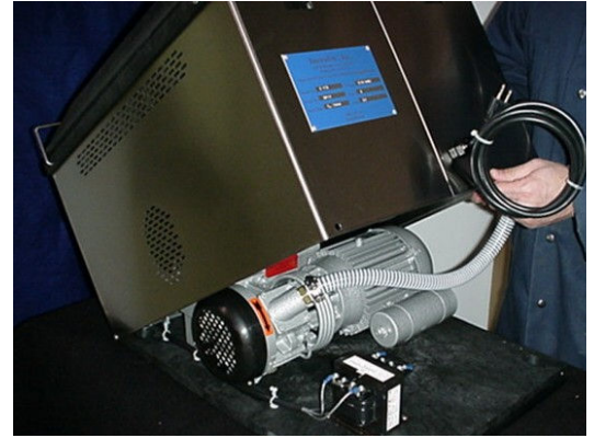
Figure 2: Remove the filler plates and sample from inside the vacuum chamber. Cushion the front of unit with a pad and lift up and forward.
