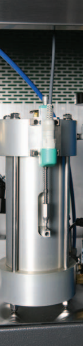
Above: Combined pressure / volume-change apparatus
